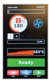
When the oven is at the correct temperature the ready screen will show.
