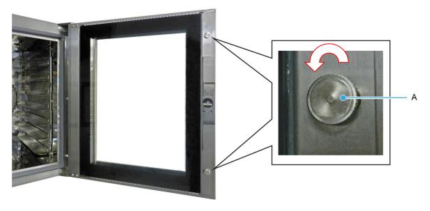
A. Undo the two screws to release the inner glass for cleaning
