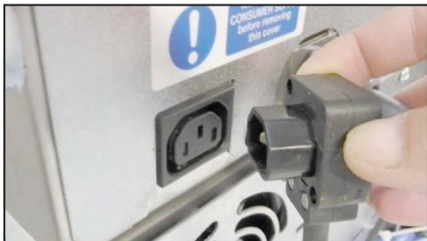
Figure 46: Plugging in the condenser unit
