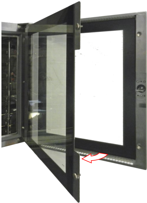
Figure 7: Inner glass panel moved away from the door
