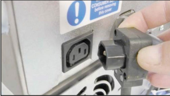
Figure 45: Plugging in the condenser unit
